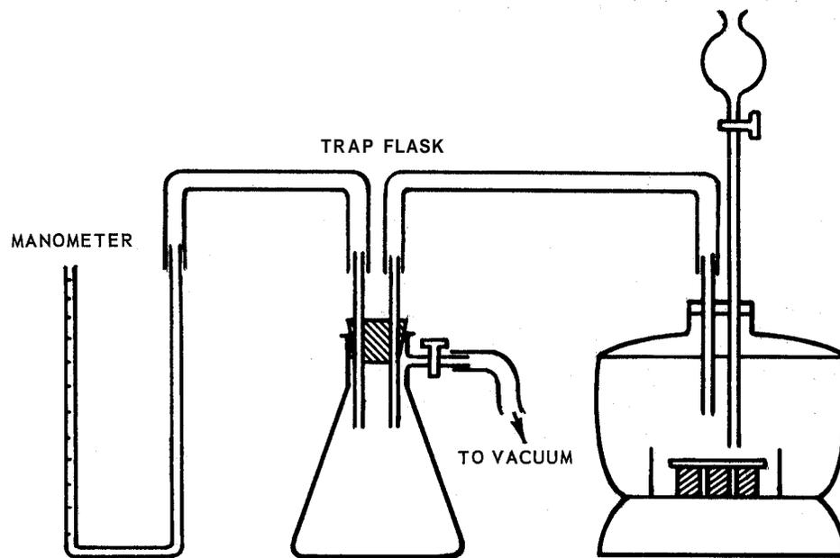
FIGURE 1. IMPREGNATION APPARATUS
